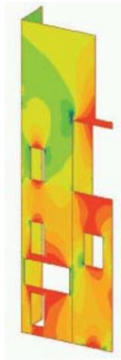
14. Detailed finite element model.
